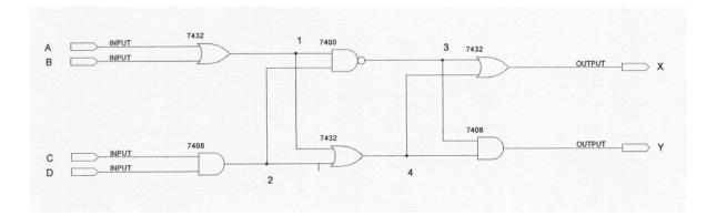
1. Define the path from input to output and identify the nodes (indicated 1, 2, 3 and 4 on the schematic) constituting the critical path. Be sure to take inversions into account when determining the maximum propagation delay.
